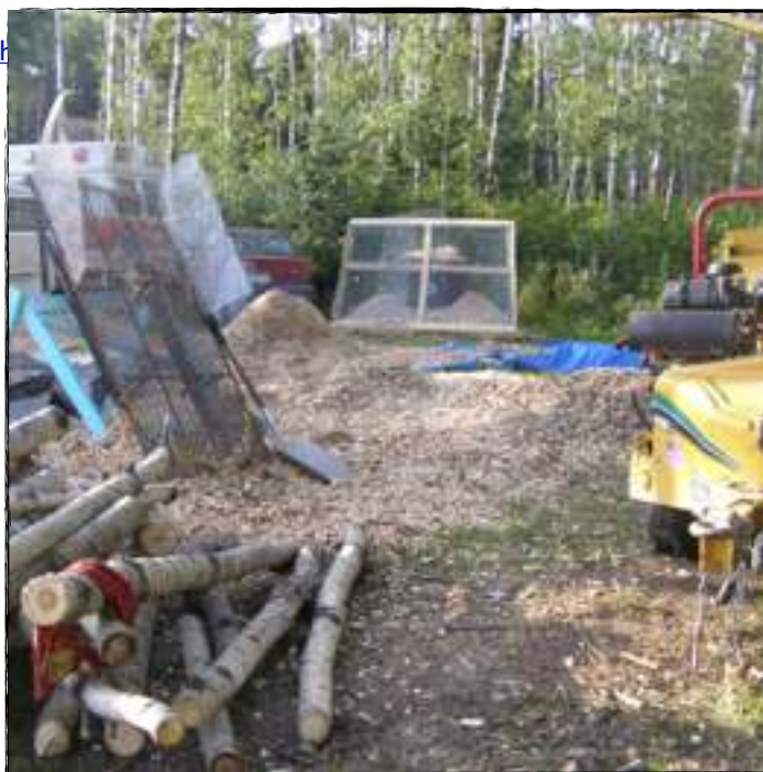
RIGHT. A Vermeer BC 600 Disk Chipper. LEFT, you see a primary screen filter, which all chips were blown against to remove the fines. In the background, you see the large screen that was used to filter out anything less than 1 cm (1/4 inch hardware cloth was used.)
