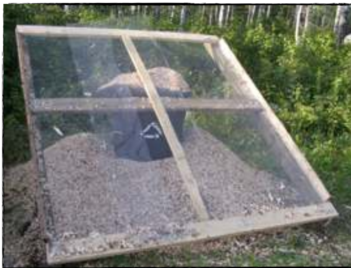
A close up of the homemade sorting/sifting screen. Chips are loaded onto the screen and it is shaken to allow the larger chips to fall onto a collection tarp at the bottom, while fines fall through.
