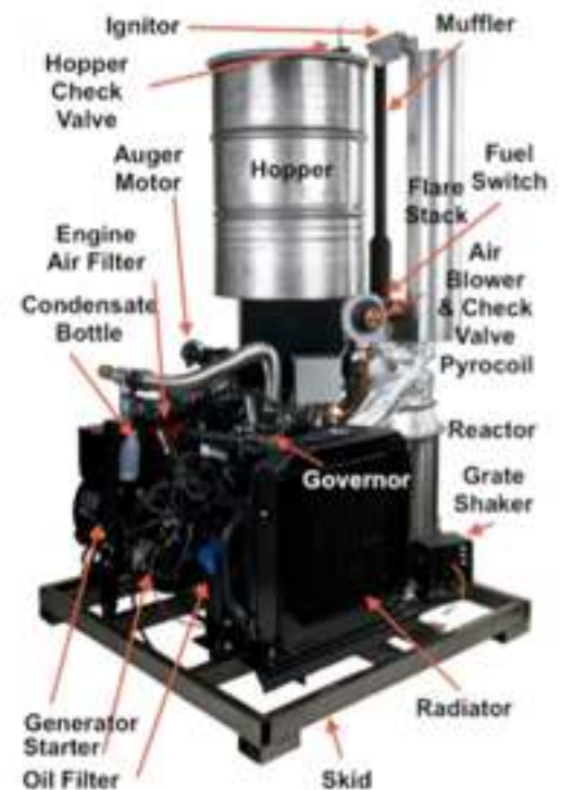
The components of the GEK Gasifier.
