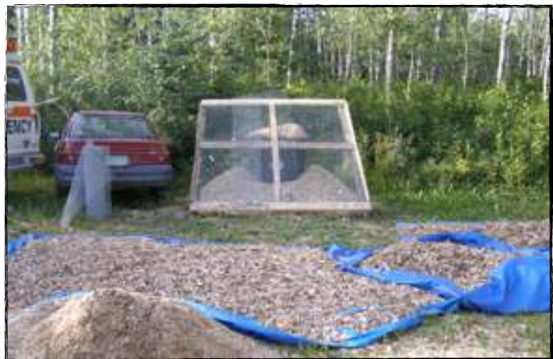
All chipped material was loaded onto this screen built of 1/4" hardware cloth. Shaking & banging it filtered out all fines and the finished material
